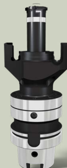
Internal and external boring with grooving by use of interpolation.
